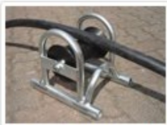
Cable laying roller with fibre glass reinforced polyamid roller body high steel frame: clearance under the roller 160 mm low steel frame: clearance under the roller 100 mm
